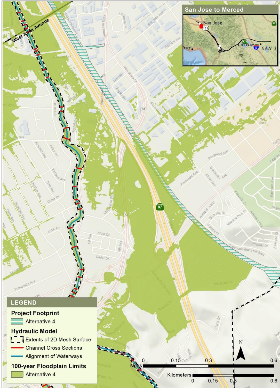
Figure 4-15 100-Year Floodplain at Almaden-Curtner Area from Hydraulic Analysis, Alternative 4
