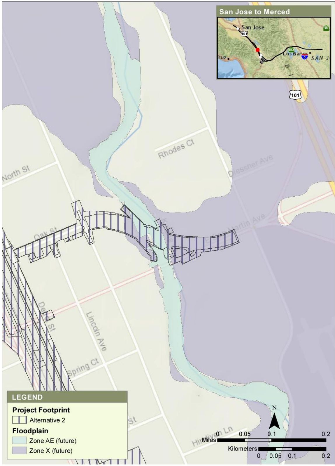
Figure 3-30 Llagas Creek (at East San Martin Avenue), Floodplain after Completion of Upper Llagas Flood Protection Project with Project Footprint for Alternative 2
