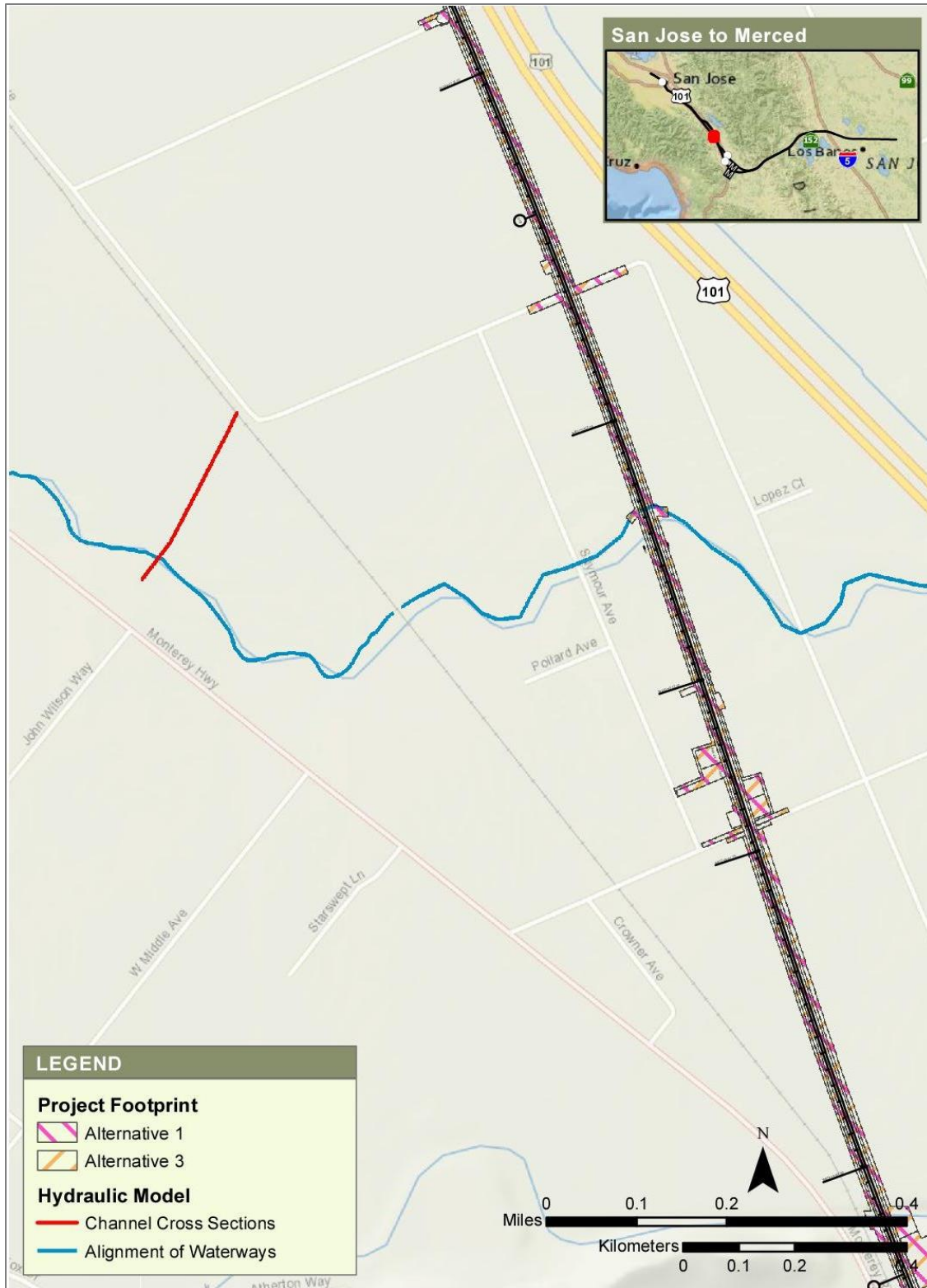
Figure 3-15 West Little Llagas Creek, Plan View of FEMA Effective Hydraulic Model with Project Footprint for Alternatives 1 and 3
