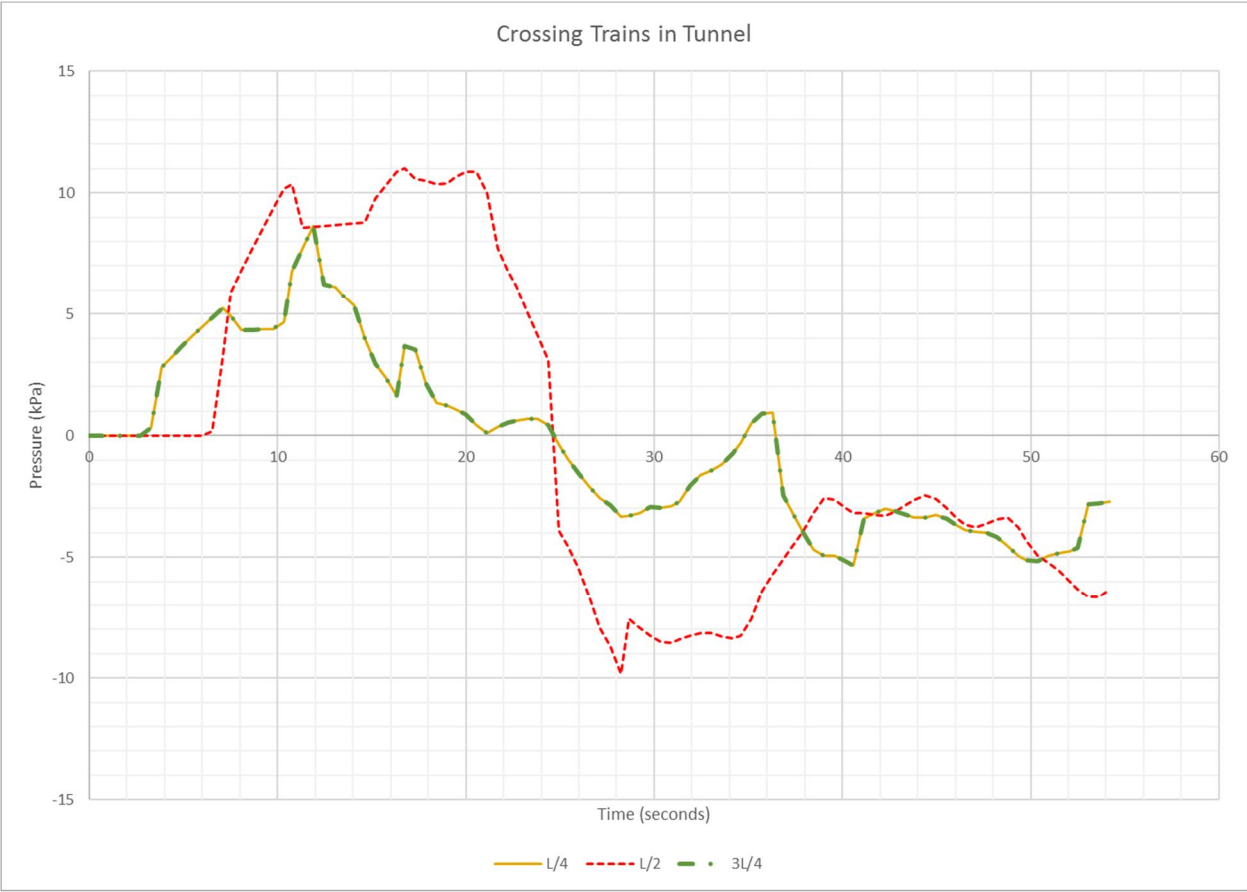
Figure 5: Pressure in the Tunnel
