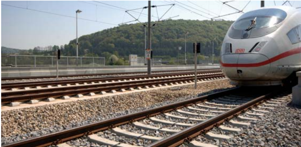
Figure 4-13 Ballast Track - Schotteroberbau
