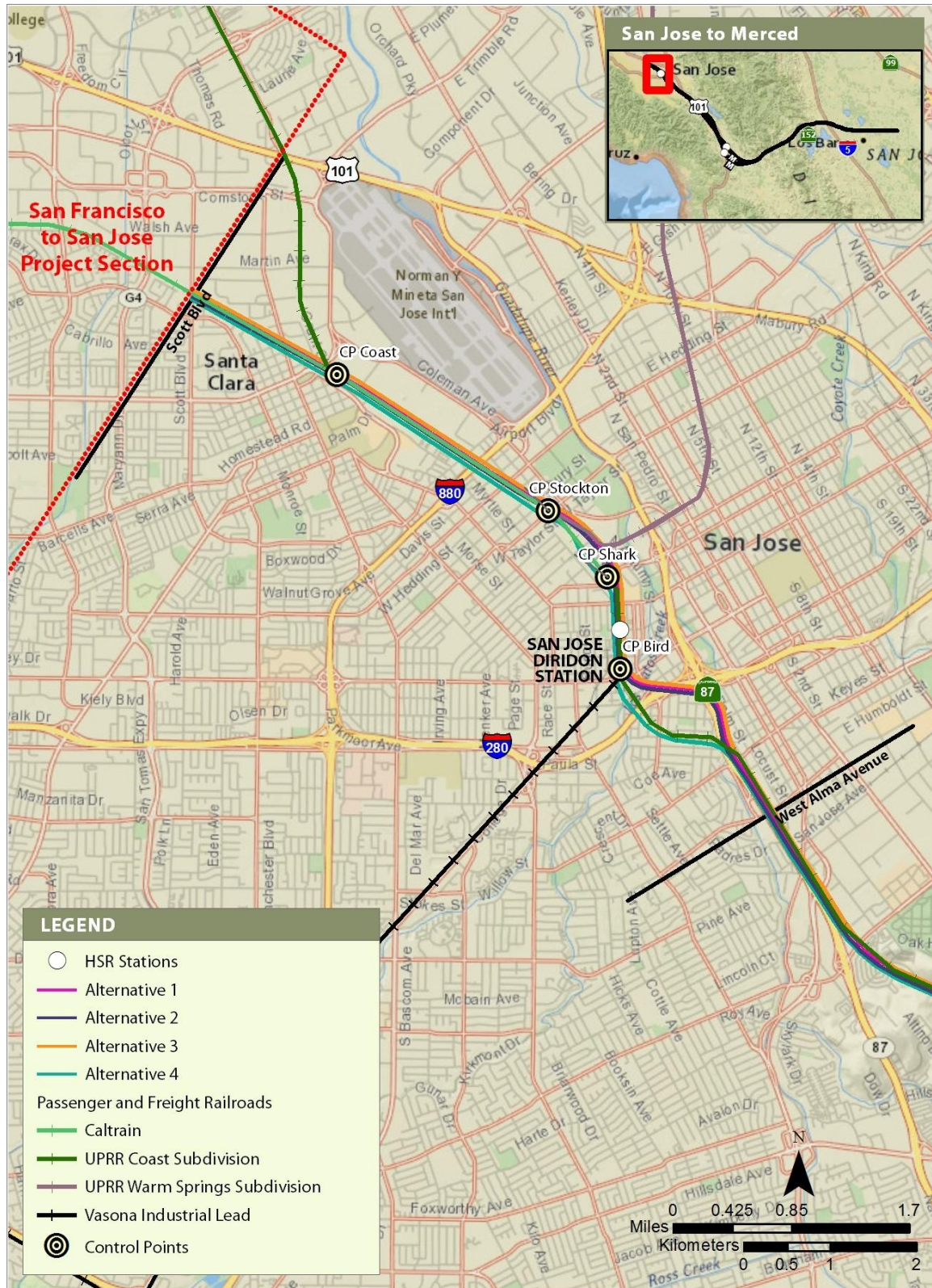
Figure 3.2-9 Railroad Control Points and Subdivisions in the RSA (San Jose Diridon Station Approach Subsection)
