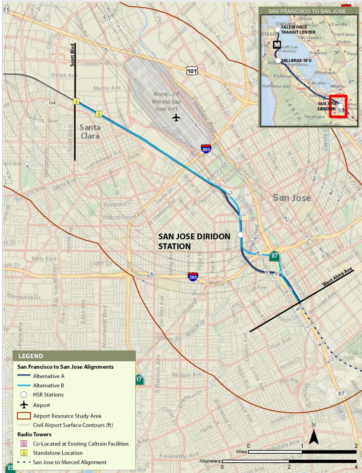
Figure 6 Part 77 Contours and Tower Locations—San Jose Diridon Station Approach Subsection
