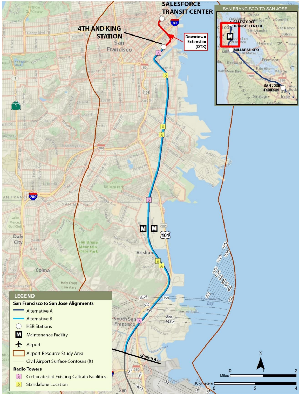
Figure 2 FAA Part 77 Contours and Tower Locations—San Francisco to South San Francisco Subsection
