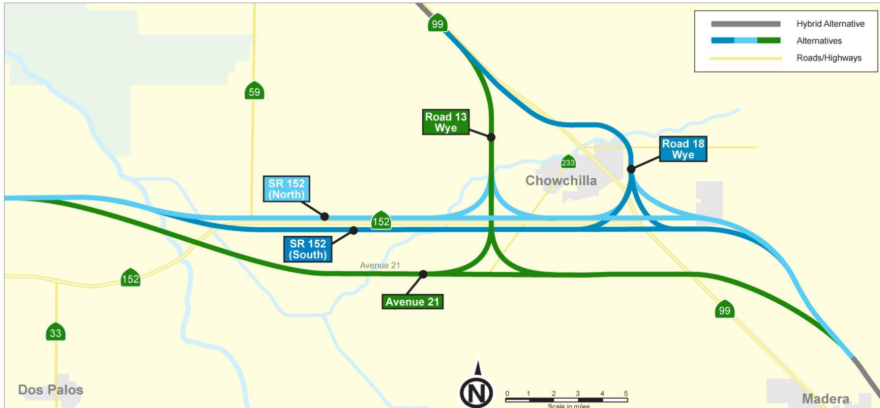
Figure 2-4 Four Central Valley Wye Alternatives Carried Forward in Supplemental Alternatives Analysis Report (April 2013)
