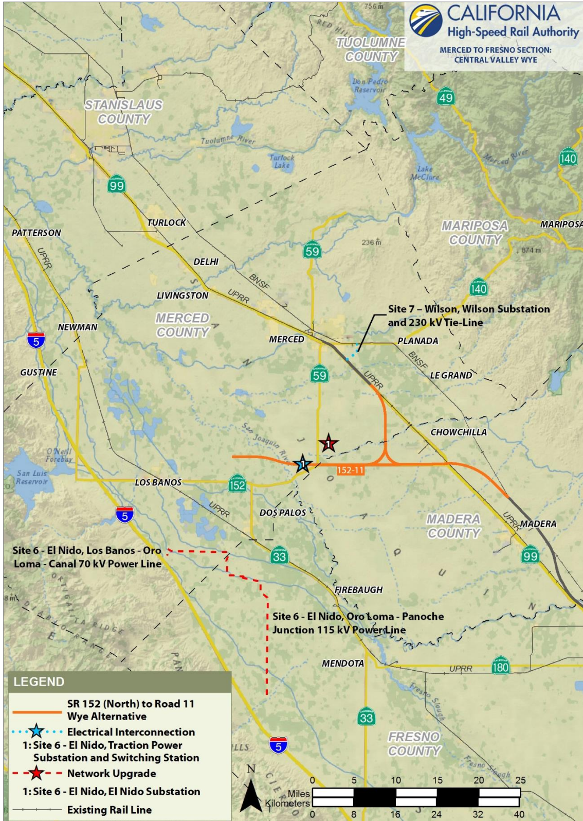
Figure 2-8 SR 152 (North) to Road 11 Wye Alternative Electrical Interconnections and Network Upgrades
