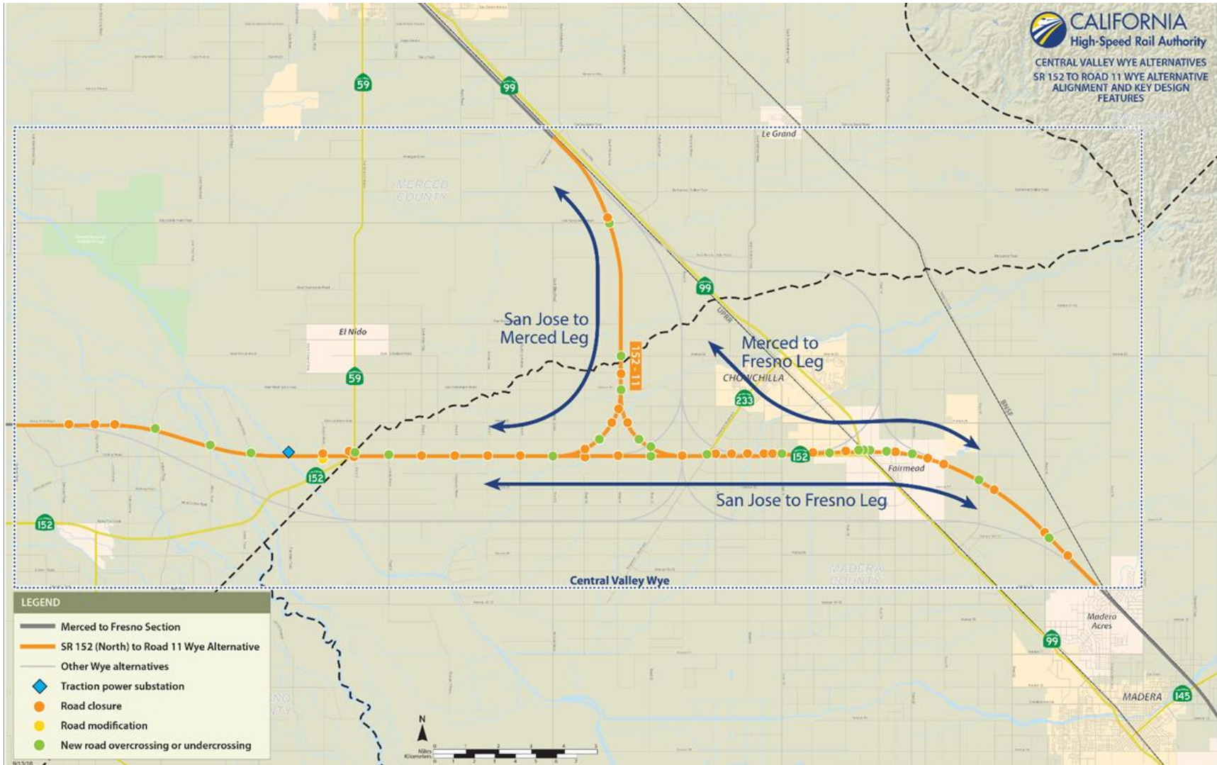
Figure 3-4 SR 152 (North) to Road 11 Wye Alternative Alignment and Key Design Features
