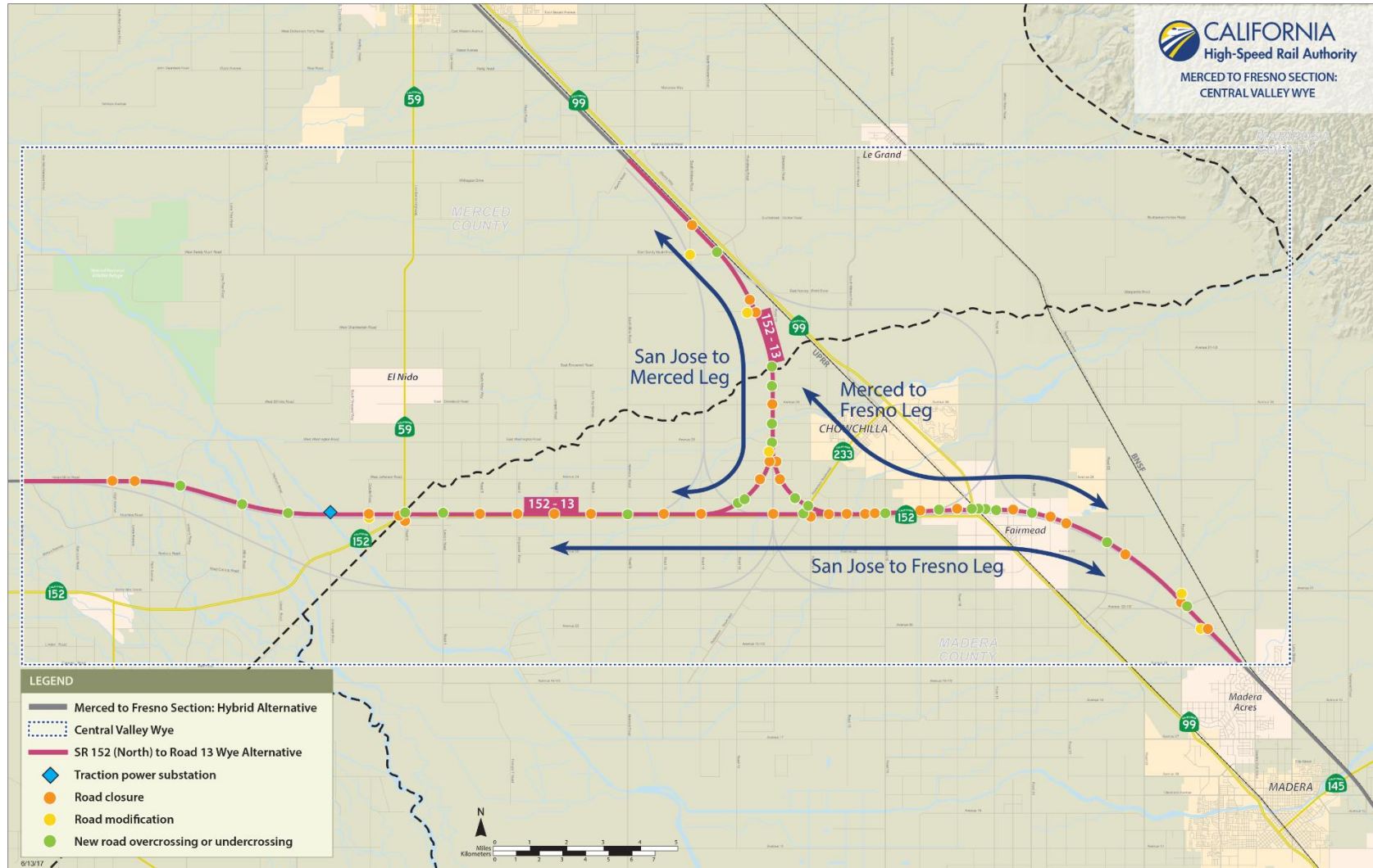
Figure 3-1 SR 152 (North) to Road 13 Wye Alternative Alignment and Key Design Features
