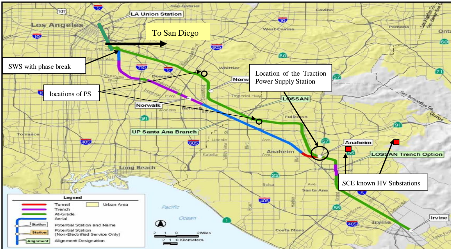
Figure 6: Feeding configuration between Los Angeles and Anaheim used for the traction power simulation
