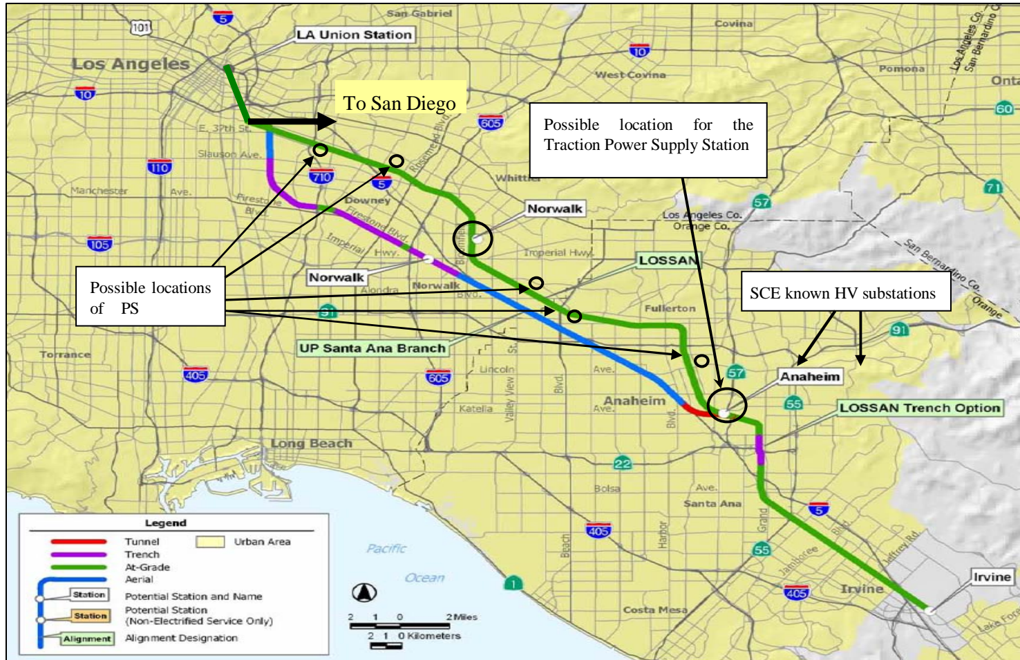
Figure 5 : Possible locations of the Traction Power Supply Station and Paralleling Stations between LA and Anaheim
