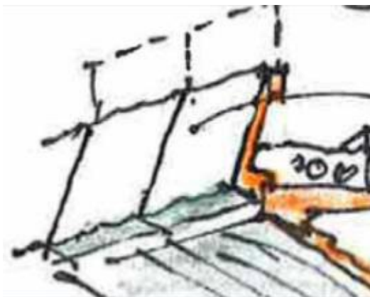
Sound Wall/ Parapet for Angled Girder
