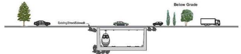
Figure 2 Typical Section for Below-Grade Option
