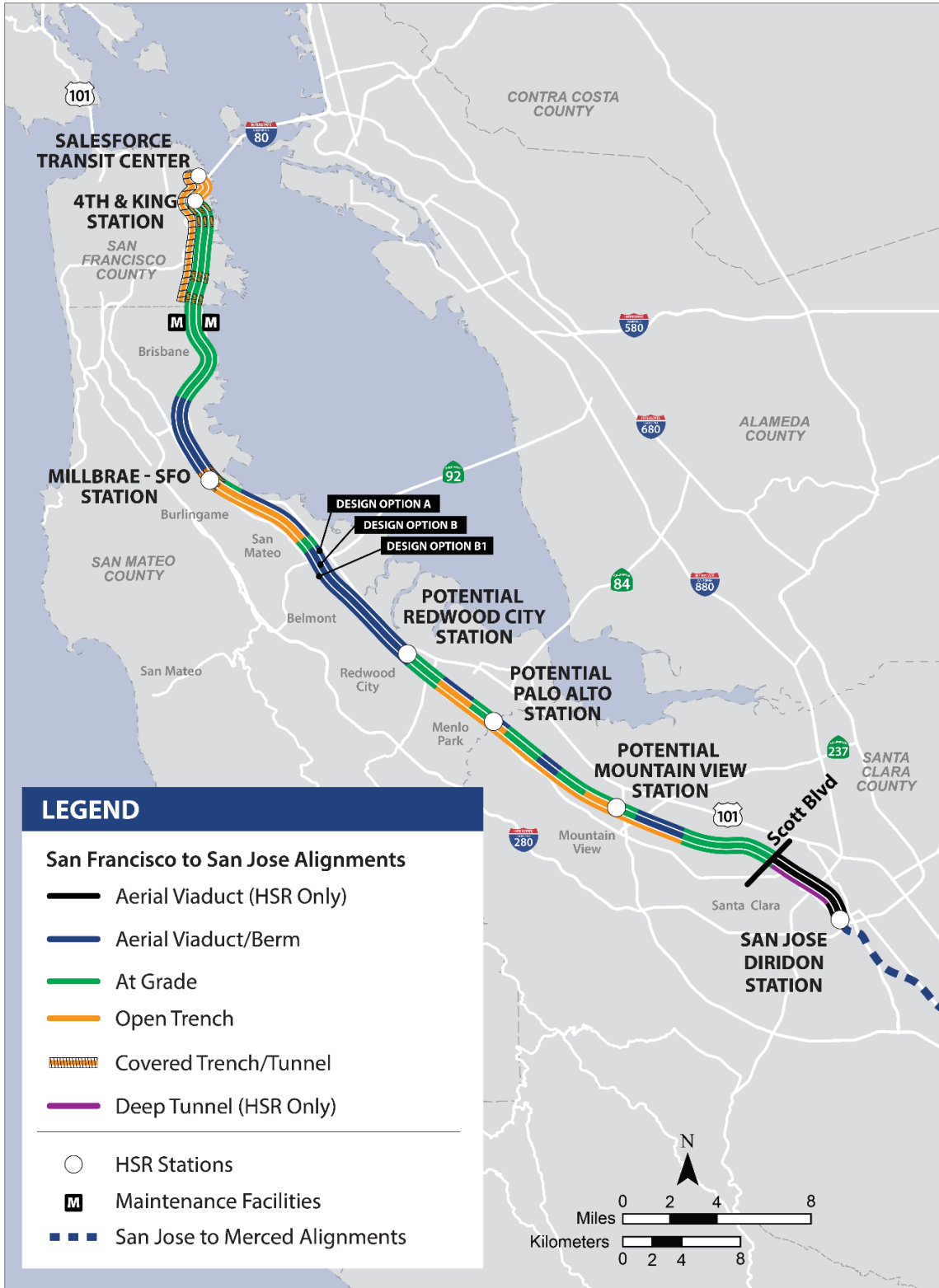
Figure 5 Alignment Alternatives, Station Locations, and Light Maintenance Facilities Carried Forward from the Supplemental Alternatives Analysis
