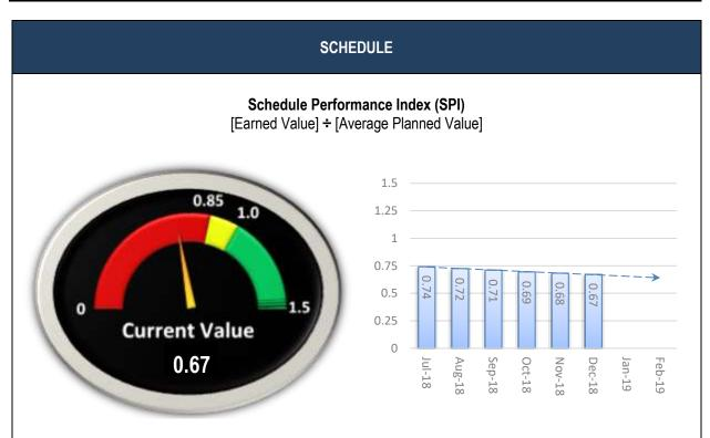
**Reason** – September 2017 the methodology used to perform the SPI calculation was revised to more accurately reflect progress (earned value) regarding the Contractor's plan (planned value). Previously, change orders executed after approval of the baseline schedule were skewing the calculation. This adjustment resulted in a reduction of the earned value portion of the calculation, and correspondingly, a lower SPI.
