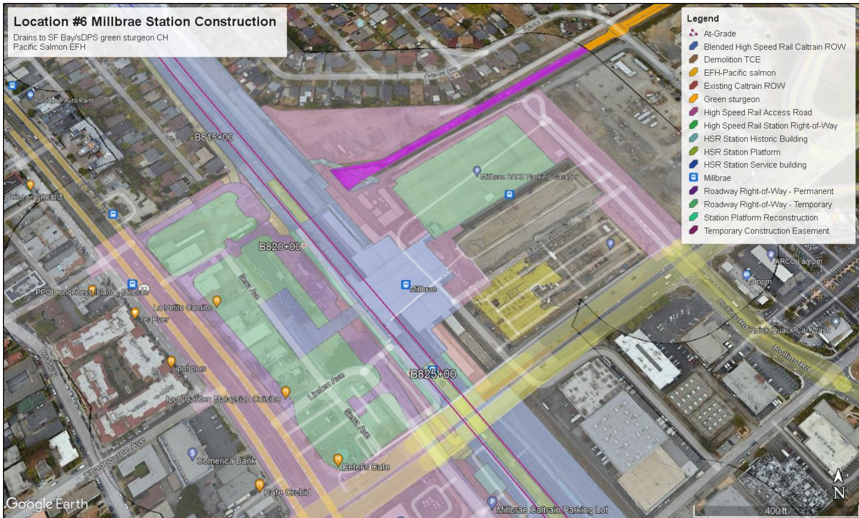
Figure 9. Millbrae Station Location #6. HSR to use existing at-grade tracks (maroon lines) to service existing Millbrae BART Station. Areas to be altered in station redesign represented by multiple opaque layers. Highline Creek (now considered a constructed watercourse, vibrant magenta) drains to San Francisco Bay estuarine/marine waters and sDPS green sturgeon designated critical habitat (downstream of vibrant orange sturgeon layer).
