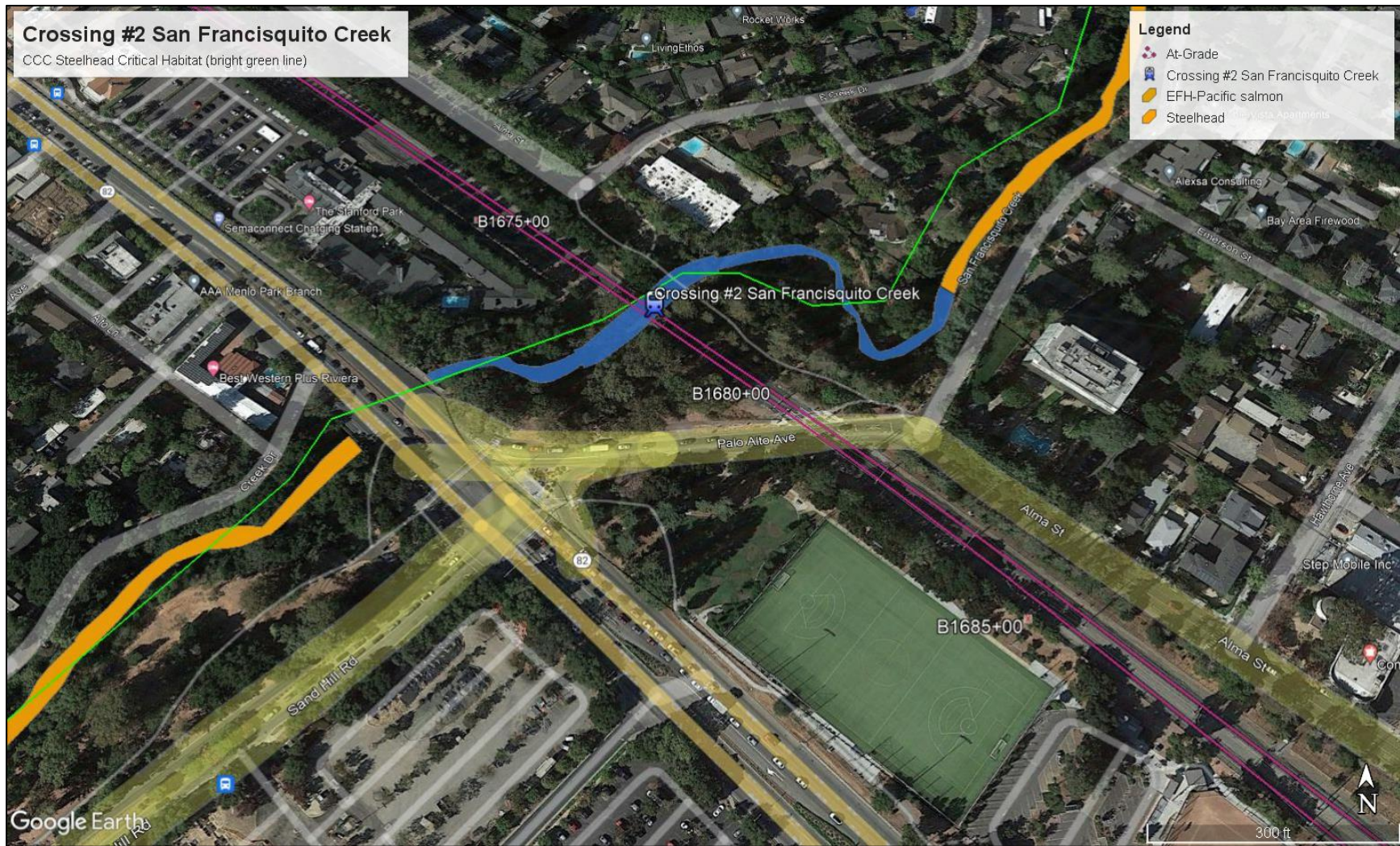
Figure 6. San Francisco Creek Crossing #2. HSR to use existing at-grade tracks (maroon lines) that cross Palo Alto Avenue and San Francisco Creek near HWY 82 in Menlo Park/Palo Alto, California. San Francisco Creek is CCC steelhead designated critical habitat (bright green line).
