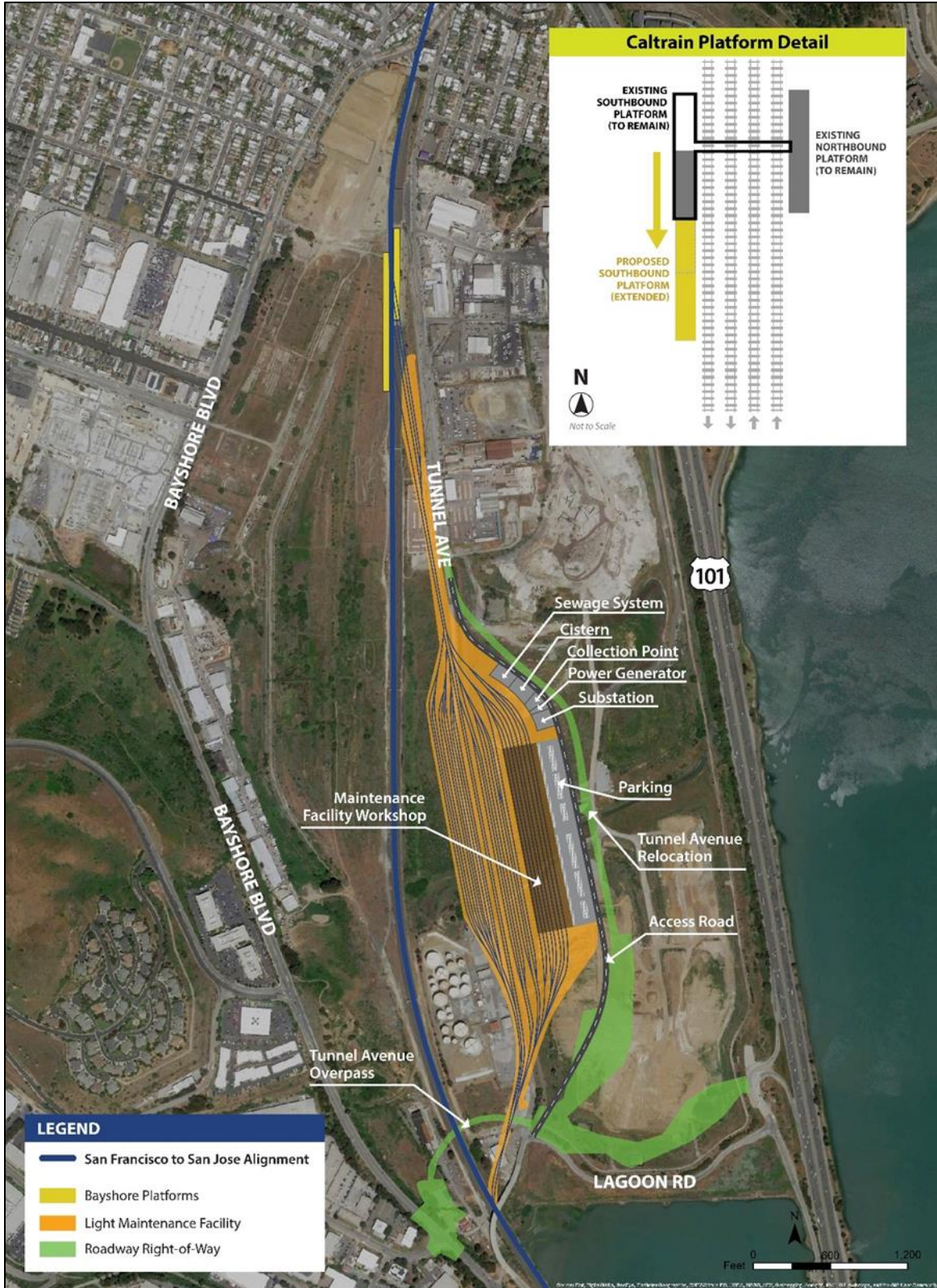
Figure 4. Proposed design of new East Brisbane LMF and Tunnel Avenue reroute and new overpass (Authority 2021i).
