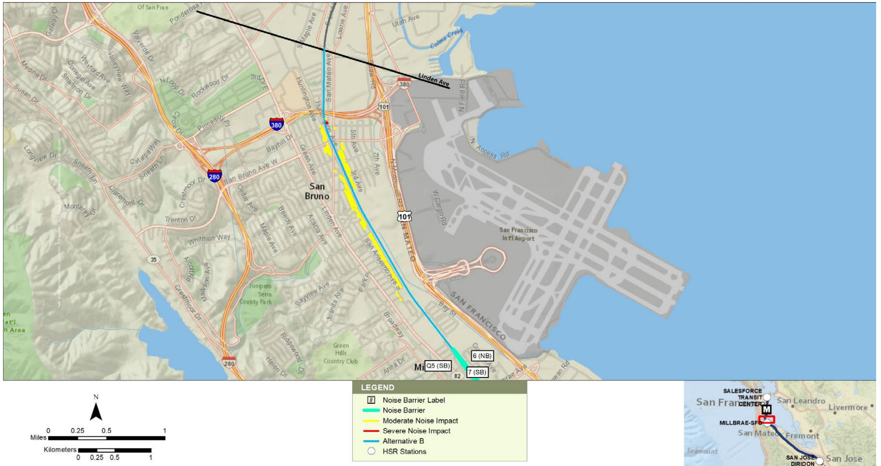
Figure C-101 2040 Plus Project Proposed Noise Barriers with Quiet Zones and Residual Noise Impacts—Alternative B
