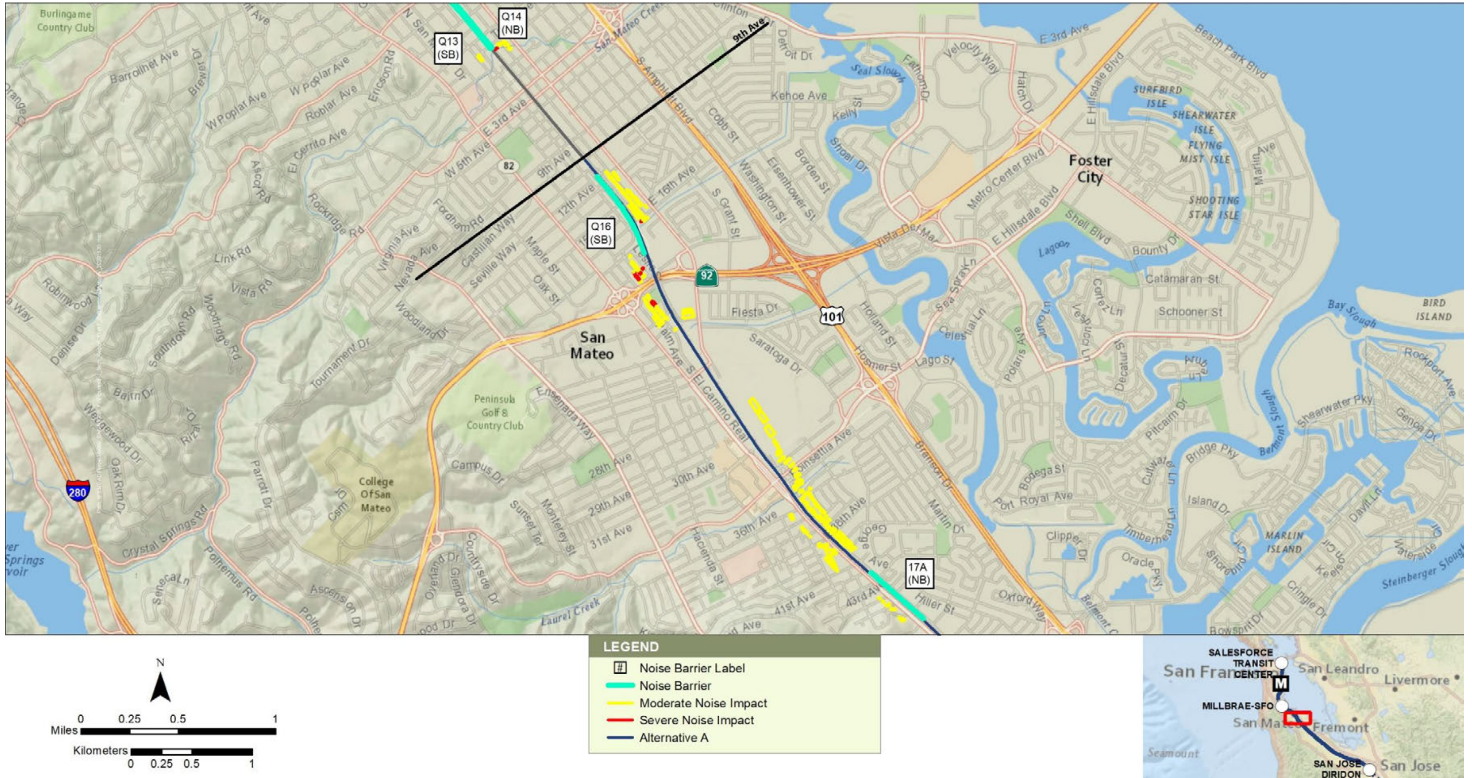
Figure C-88 2040 Plus Project Proposed Noise Barriers with Quiet Zones and Residual Noise Impacts—Alternative A
