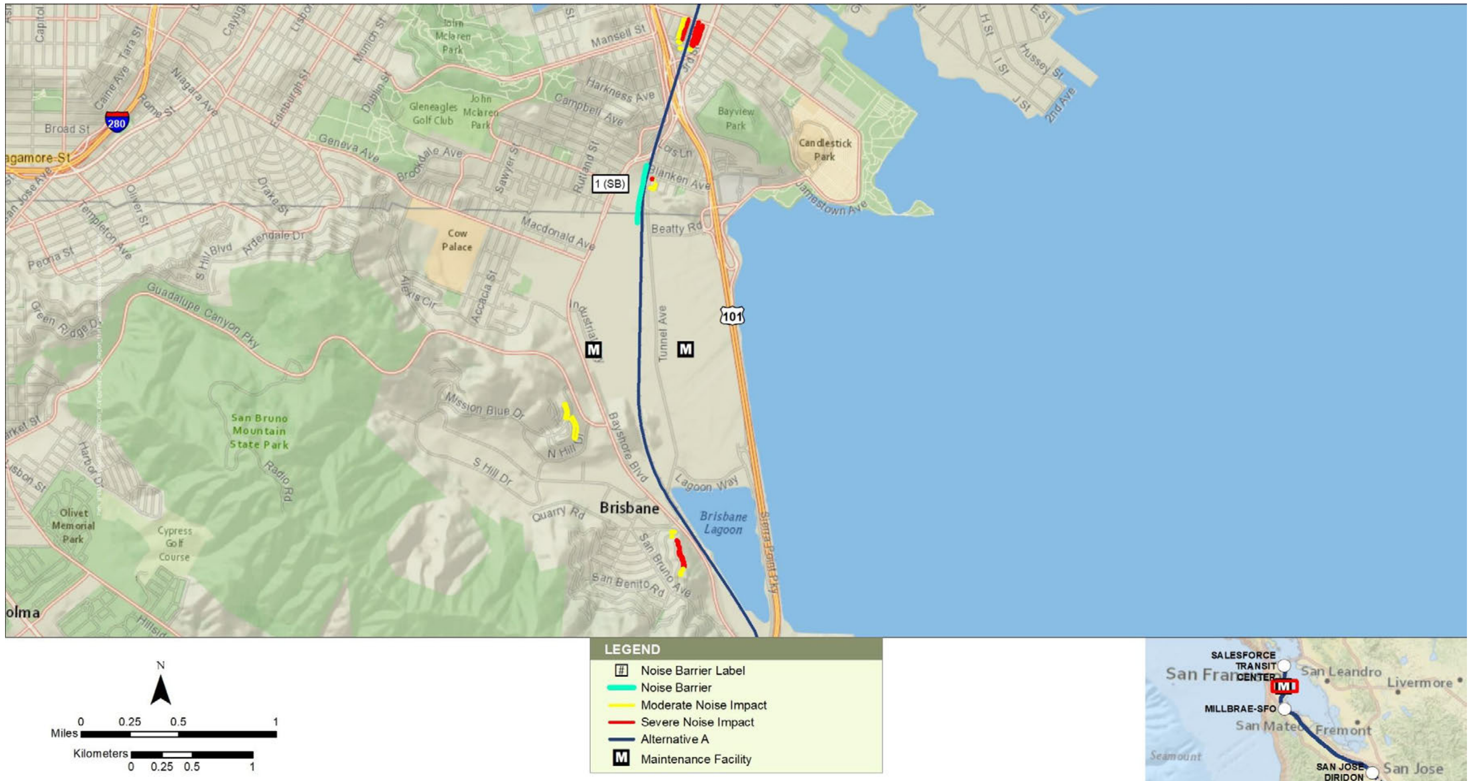
Figure C-83 2040 Plus Project Proposed Noise Barriers with Quiet Zones and Residual Noise Impacts—Alternative A
