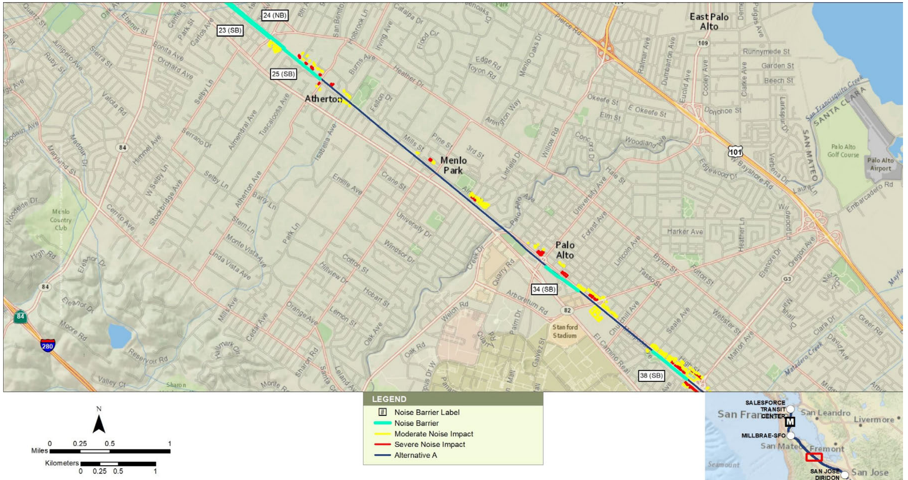
Figure C-91 2040 Plus Project Proposed Noise Barriers with Quiet Zones and Residual Noise Impacts—Alternative A
