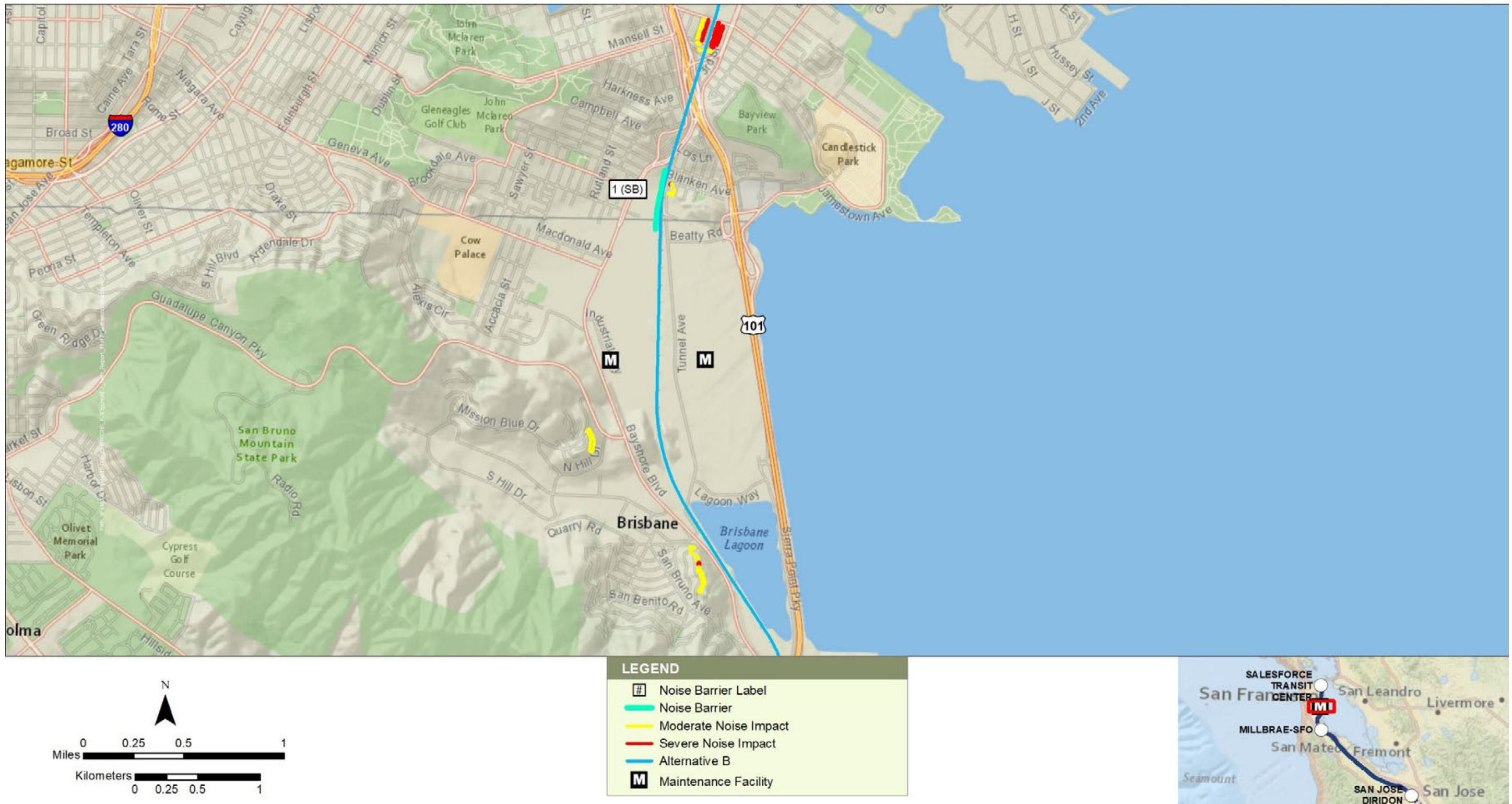
Figure C-99 2040 Plus Project Proposed Noise Barriers with Quiet Zones and Residual Noise Impacts—Alternative B
