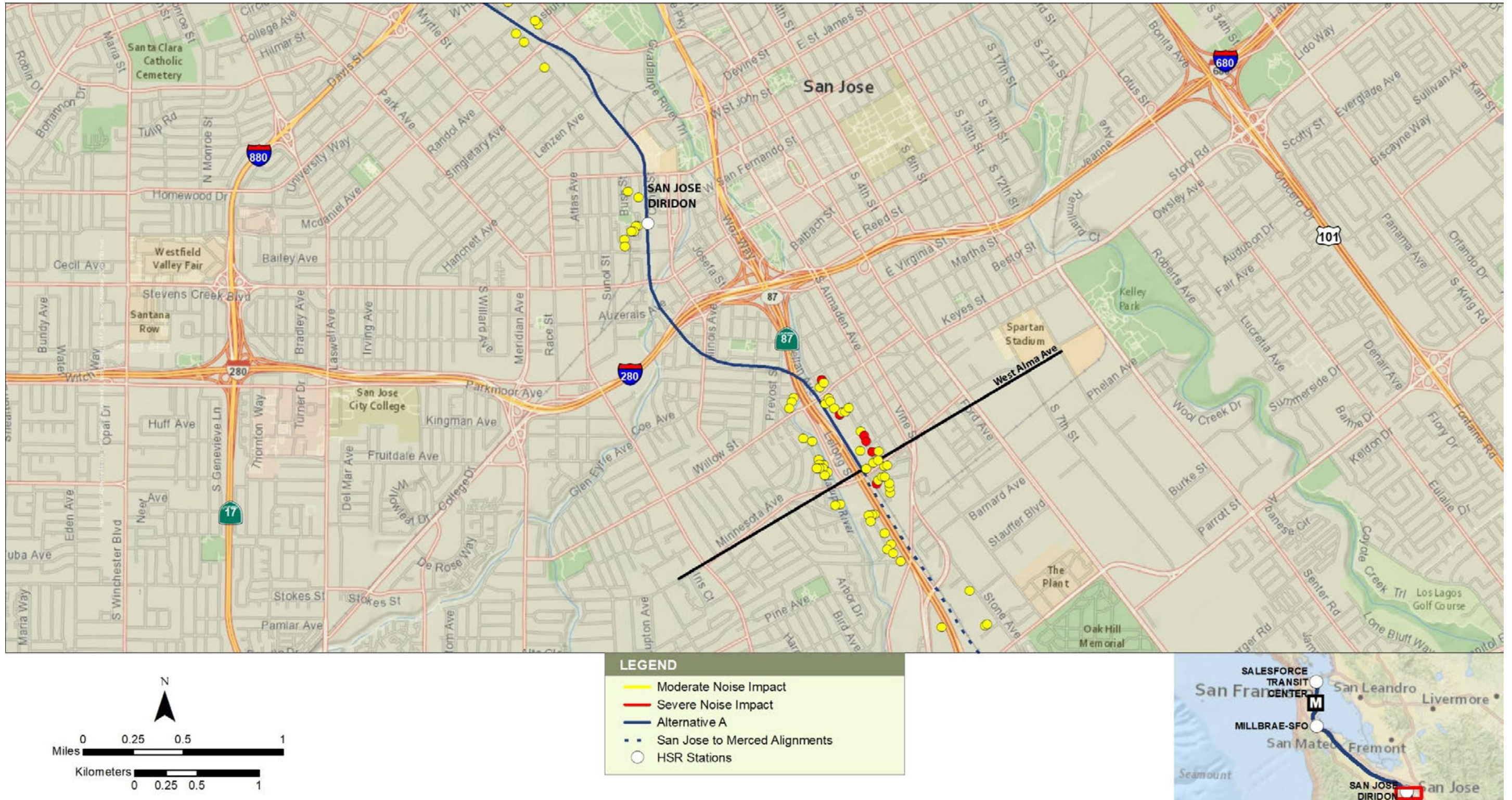
Figure C-96 2040 Plus Project Proposed Noise Barriers with Quiet Zones and Residual Noise Impacts—Alternative A
