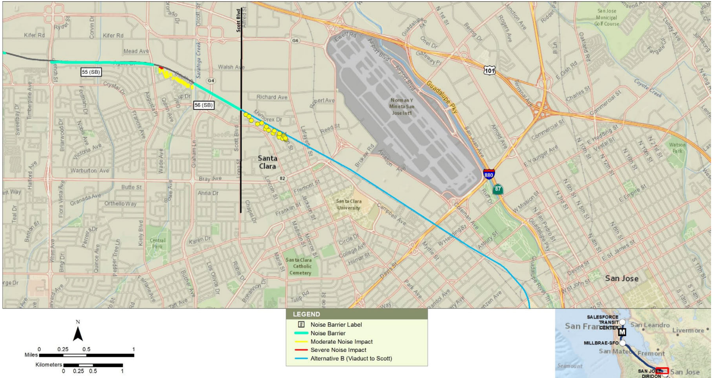
Figure C-80 2040 Plus Project Proposed Noise Barriers and Residual Noise Impacts—Alternative B (Viaduct to Scott Boulevard)
