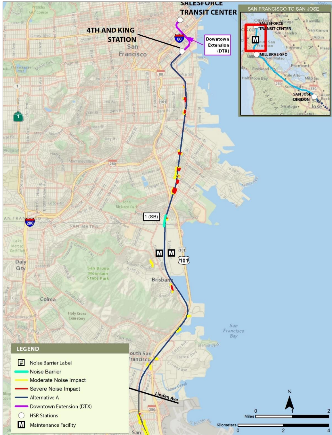
Figure 3.4-44 Noise Barriers and Residual Noise Impacts with Quiet Zones—Alternative A (San Francisco to South San Francisco Subsection)
