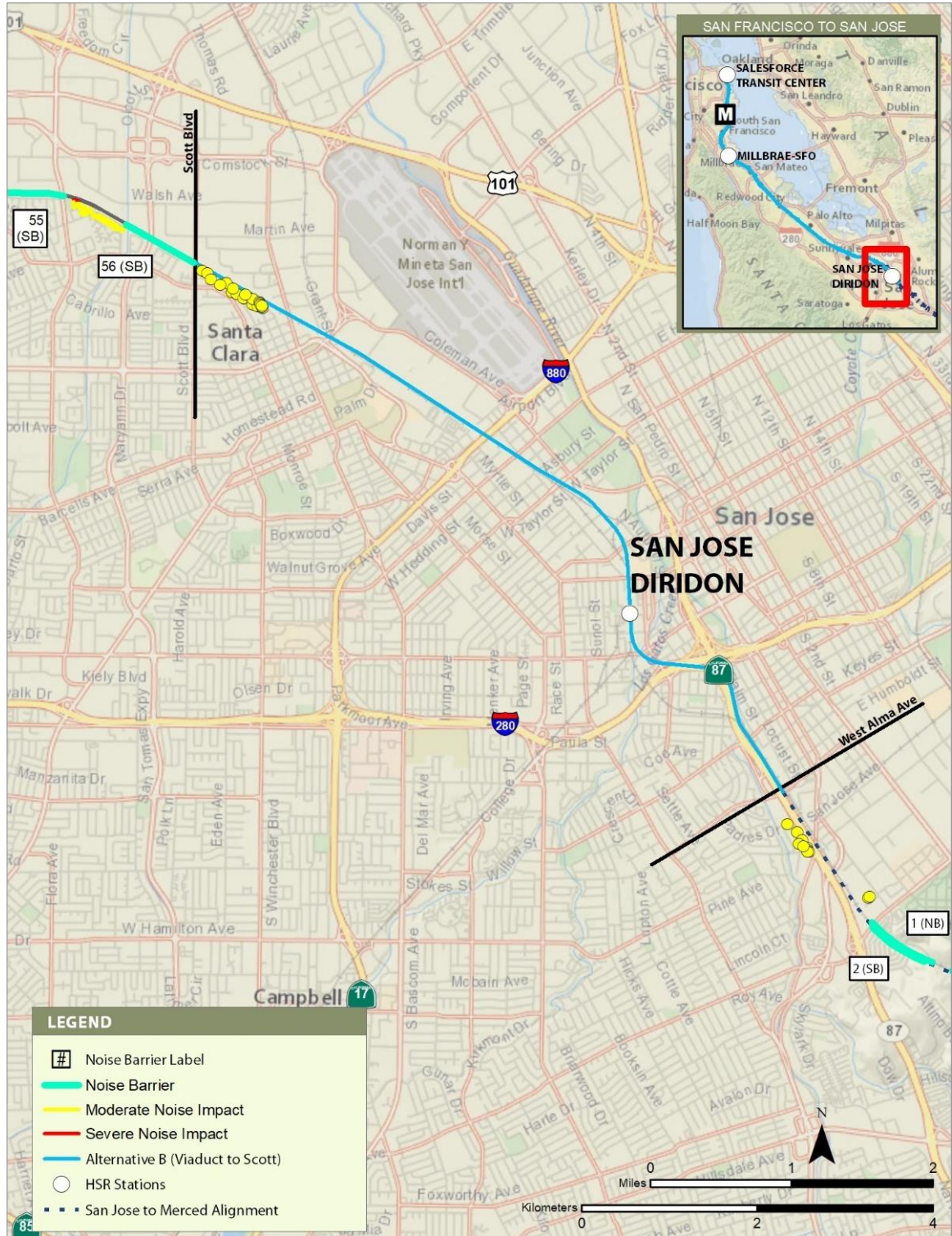
Figure 3.4-55 Noise Barriers and Residual Noise Impacts with Quiet Zones—Alternative B (Viaduct to Scott Boulevard) (San Jose Diridon Station Approach Subsection)
