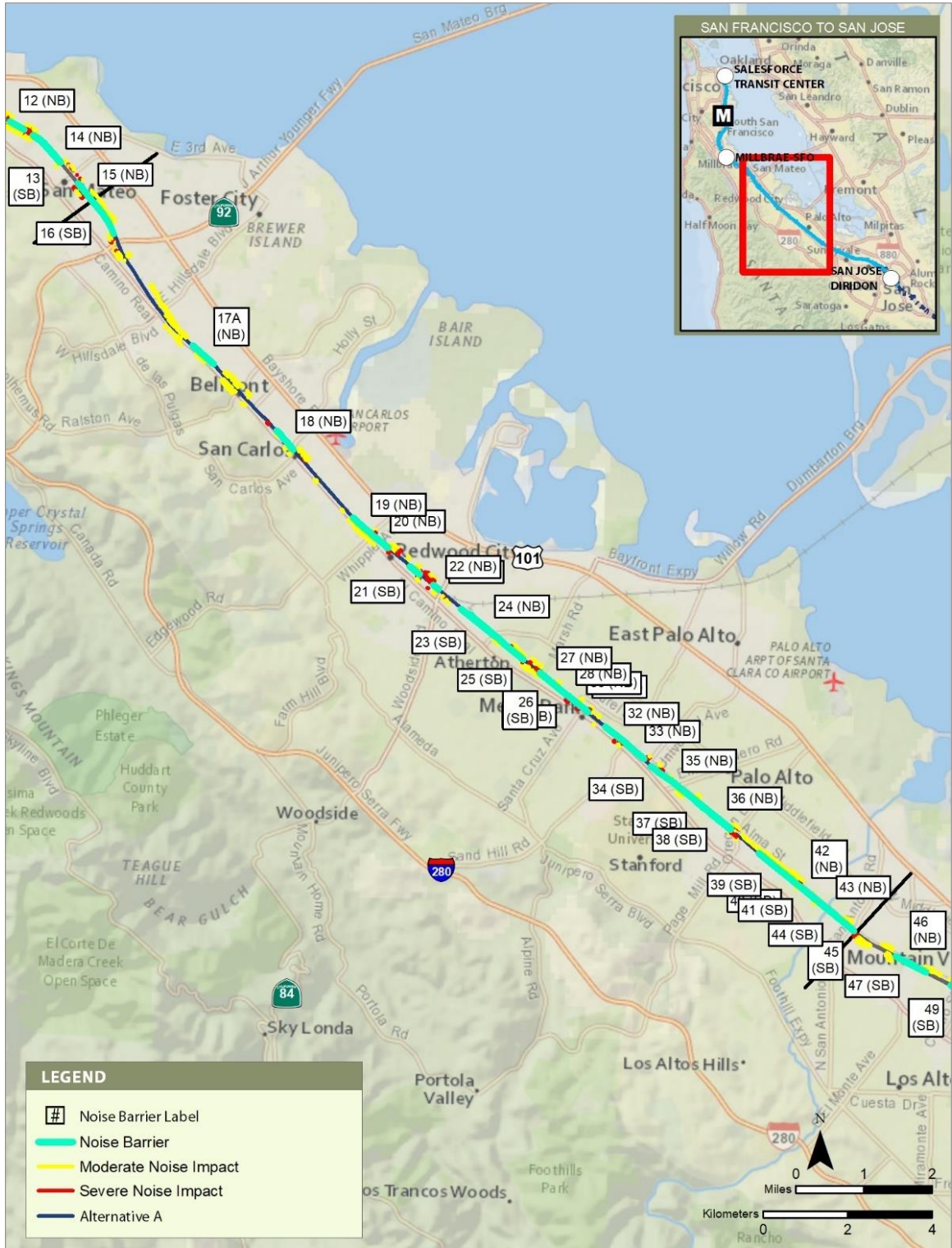
Figure 3.4-34 Noise Barriers and Residual Noise Impacts without Quiet Zones— Alternative A (San Mateo to Palo Alto Subsection)
