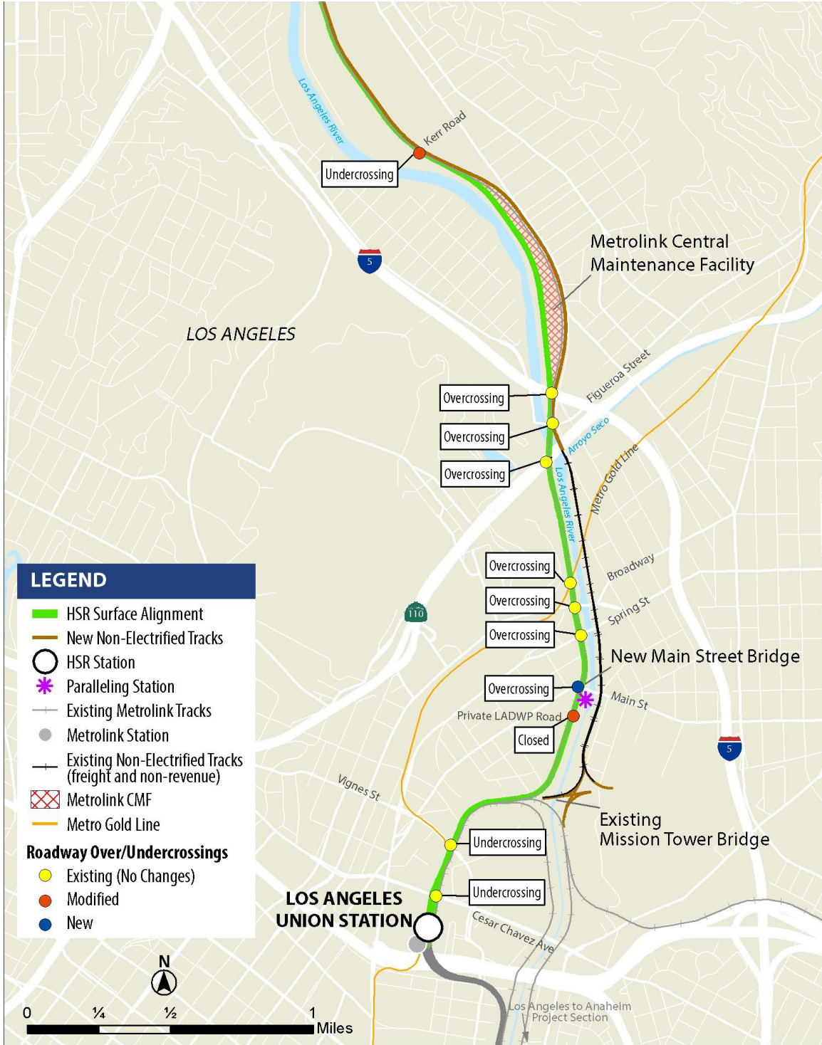
Figure 3 HSR Build Alternative Overview (Sheet 3 of 3)
