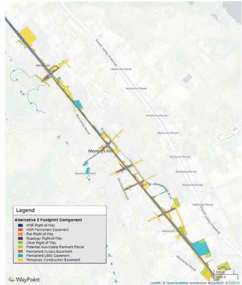
Figure 2 High-Speed Rail Alternative 2 Alignment
