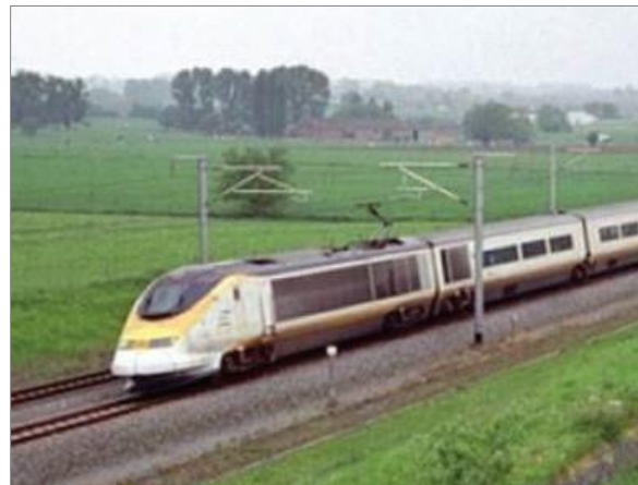
Figure 2-4 Example of an At-Grade Profile Showing Overhead Contact System and Vertical Arms of the Pantograph Power Pickups
