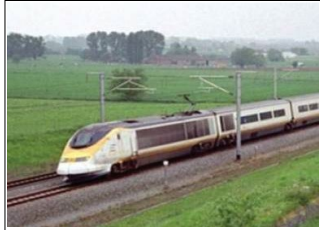
Figure 2-2 Example of an At-Grade Profile Showing Contact Wire System and Vertical Arms of the Pantograph Power Pickups
