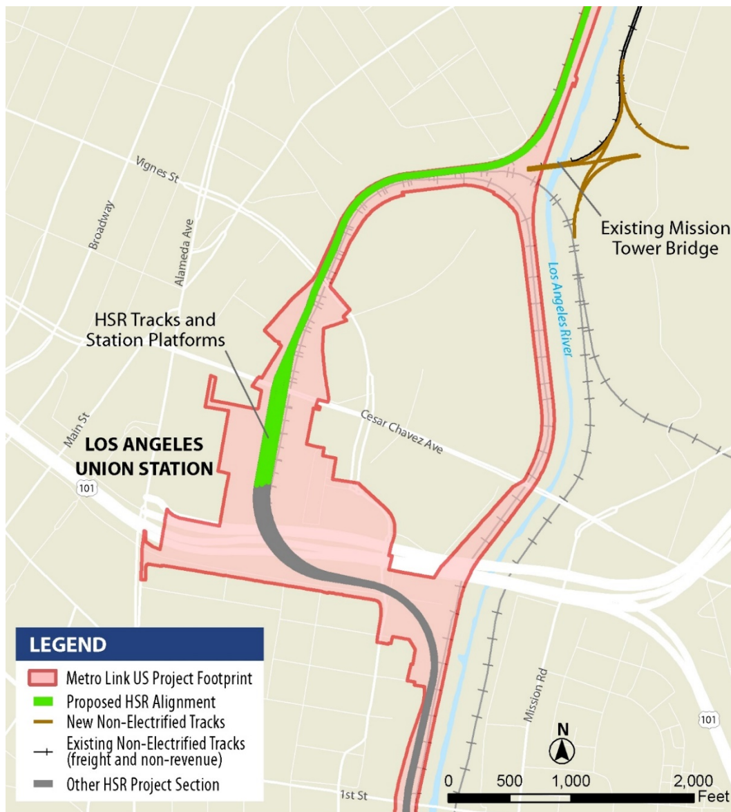
Figure 2-31 Preliminary Station Elements Plan—Los Angeles Union Station
