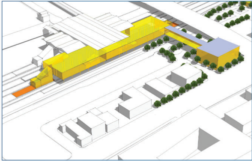
The blue represents location of Station Entrance Hall with overhead pedestrian crossing to connect high-speed rail to Caltrain and BART in the Millbrae Station Design (above) and the RSP Design Variant (below)
