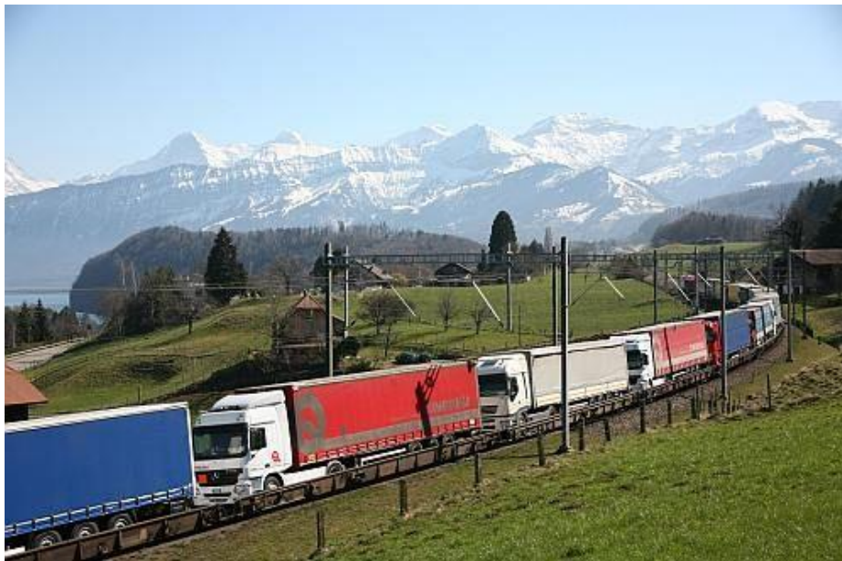
RAlpin ‘rolling road’ electric train carrying trucks in Switzerland (Photo: RAlpin AG, http://www.ralpin.ch/media/ )
